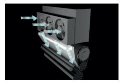
Air-blow Paper Separation Mechanism after fusing
